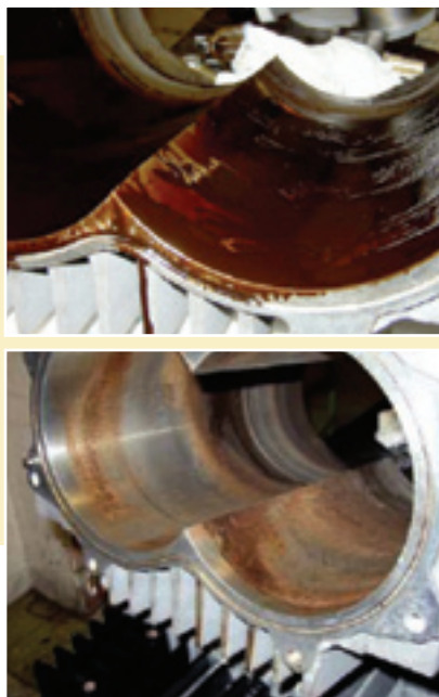
Fig. 9. Pumping chamber before and after flushing procedure
